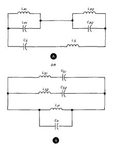
These two circuit versions fulfill this requirement. By adjusting the three L and C values, the three simultaneous resonances can be moved over a wide range.
